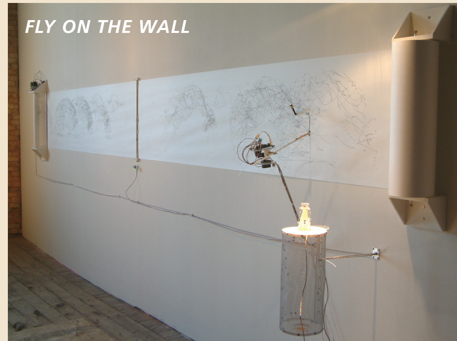
When a fly enters a chamber in David Bowen's fly drawing device, sensors detect its movement and convey the information to a microcontroller, which activates a drawing arm. The result is a sketch based on the fly's movements in real time. Once a fly is no longer detected, the drawing is complete; the paper unscrolls and a new drawing begins with a new fly.
